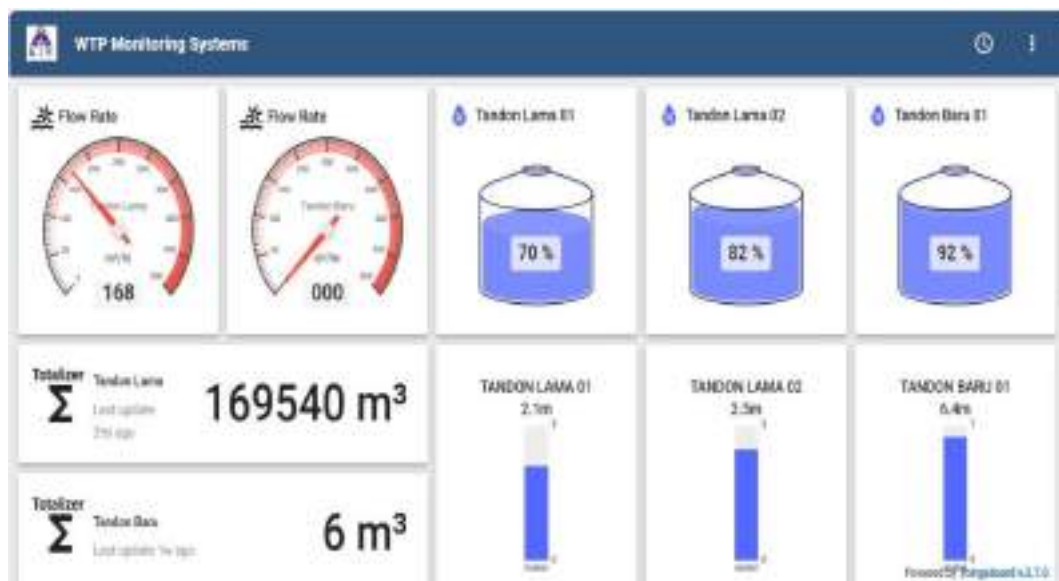
Gambar 13 Monitoring Water Meter Air Bersih & Water Level Reservoir Digitalisasi di WTP
